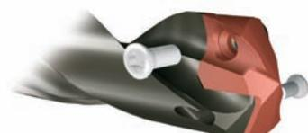
1. Place the GEN3SYS® XT Structural Steel Drill Insert into the precision ground locating pocket on the GEN3SYS® XT Structural Steel Holder.
