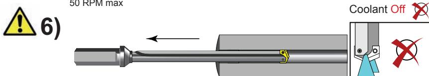
Reduce speed to a **maximum of 50 RPM** before reacting from hole
