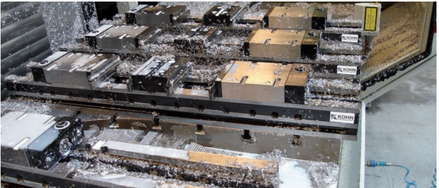
NCS 125/990 M-HD as the double vice of special funds and the second clamping jaw slide
